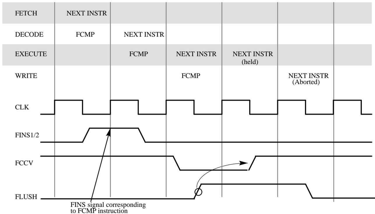
**Figure 11. Effect of FLUSH on FCMP Instruction**
