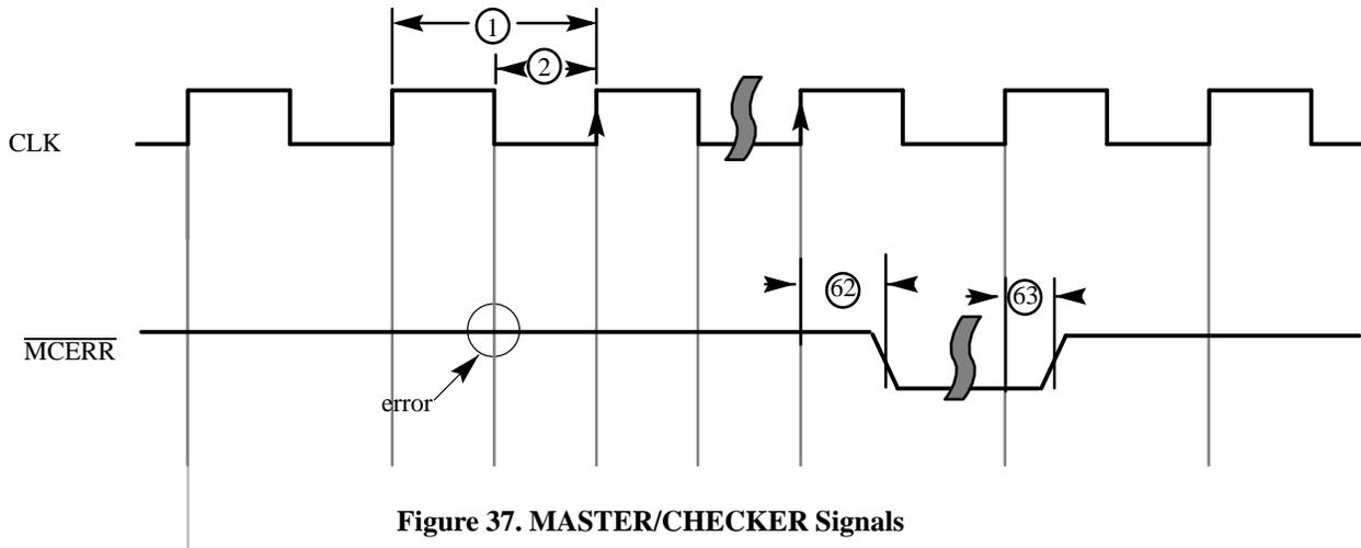
**Figure 37. MASTER/CHECKER Signals**
