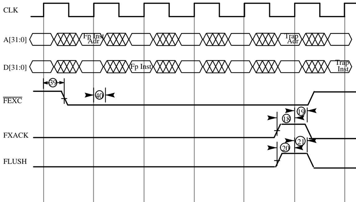
**Figure 33. Floating-Point Trap**
