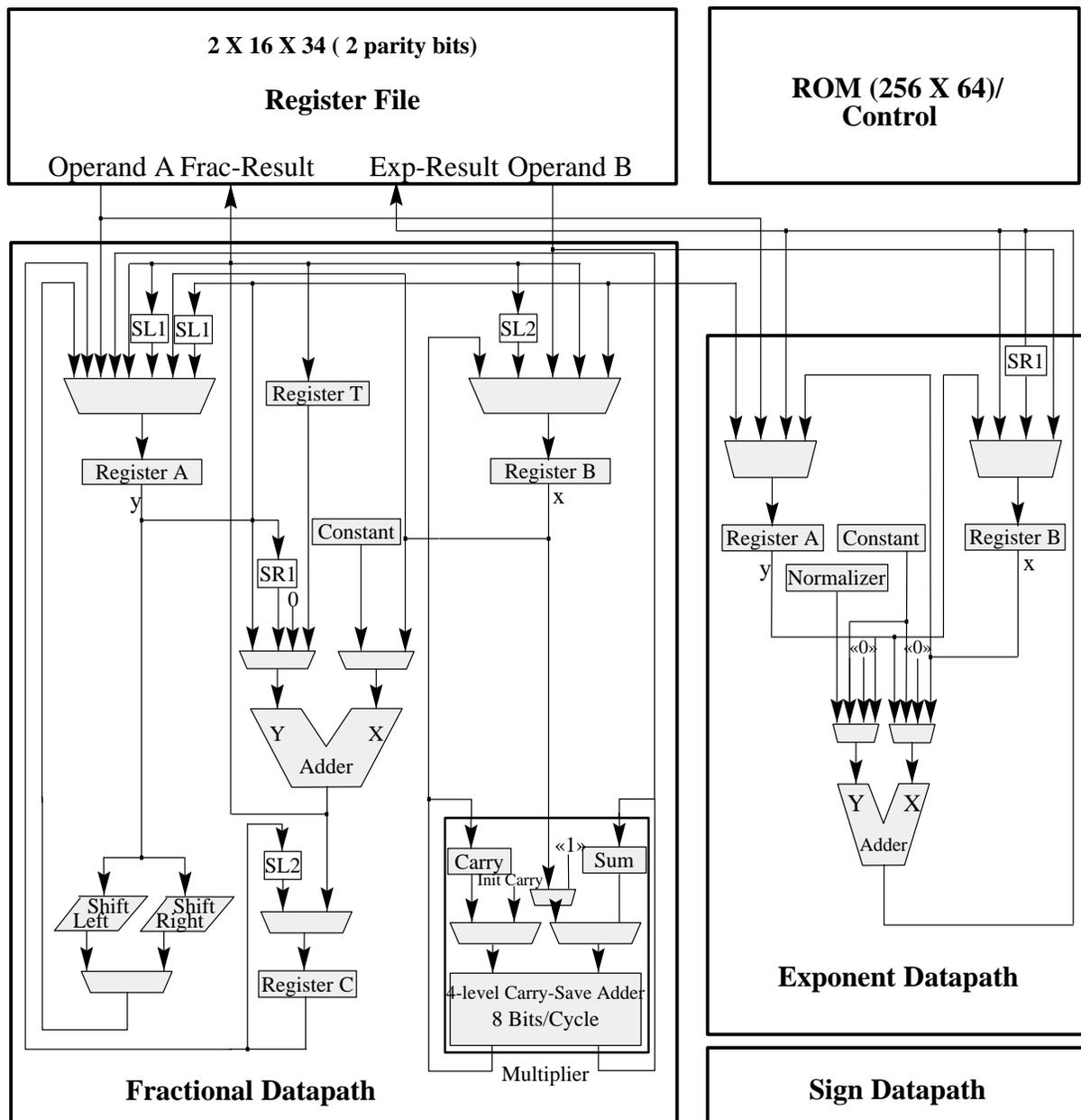
Figure 2. TSC692E Block Diagram (without parity checking)
