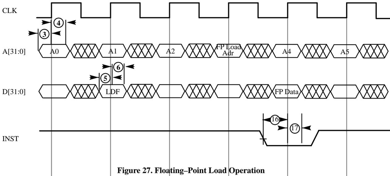
Figure 27. Floating-Point Load Operation
