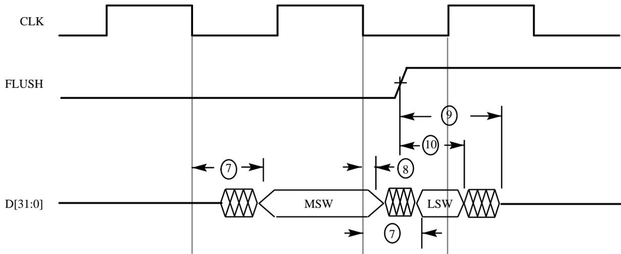
**Figure 29. Effect of FLUSH on Store Timing**
