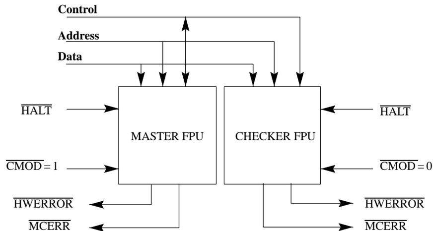
Figure 21. Master/Checker configuration
