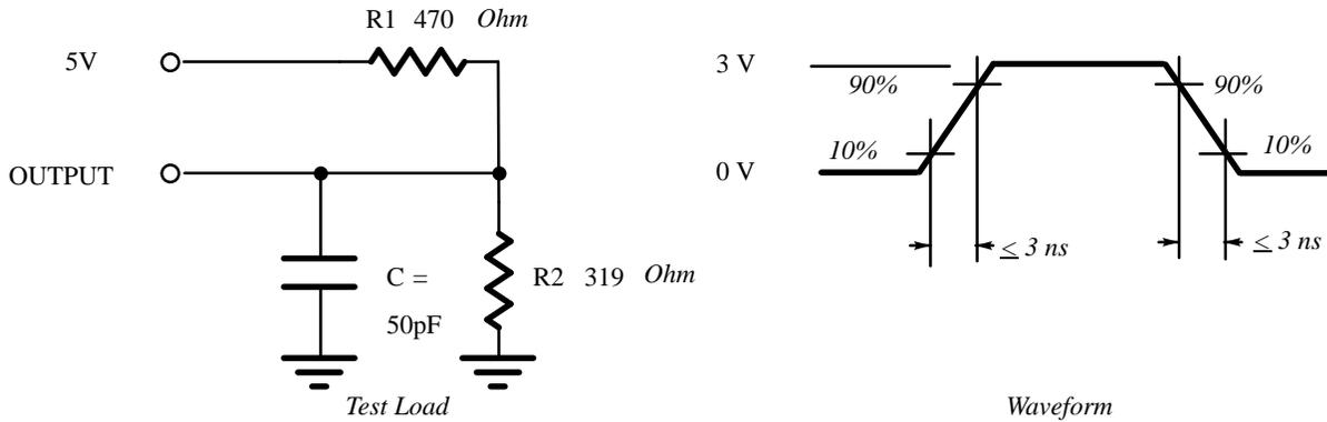
Figure 24. TSC692E AC Test Loads and Waveforms
