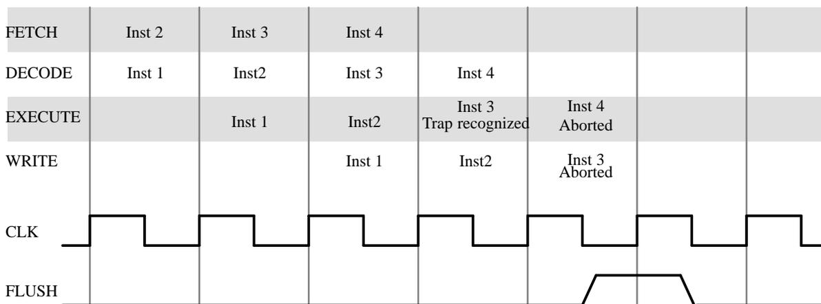
**Figure 7. Floating-Point Instruction Pipeline During A Trap**
